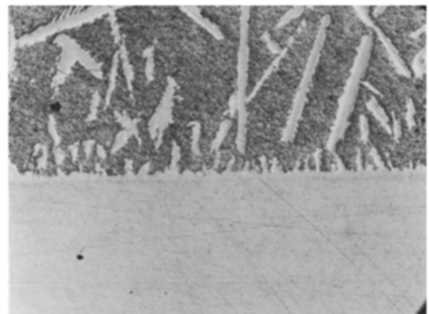
Figure 6 Cross-section through the interface formed by a tin drop and copper workpiece with an \alpha of 5.5^\circ . \times 31 .
